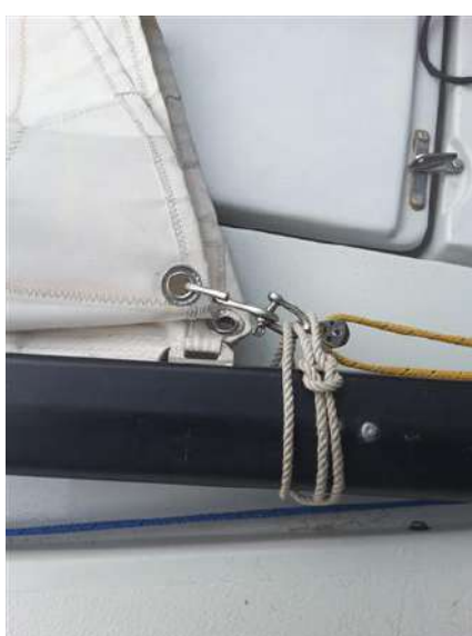
1 - Attach clew hook to leech reefing cringle 2 - Tie line around boom through shackle (not tight)
