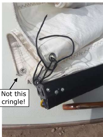
Thread a line through luff reefing cringle and around tack pin. Pull tight and knot.
