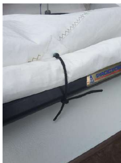
Gather up the unused sail slab with the three pairs of short lines (not tight)
